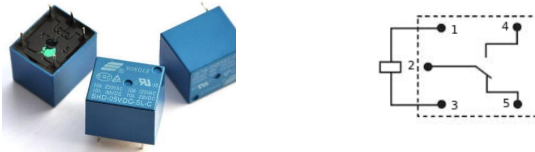
Figure.2 Relay and its pin layout
