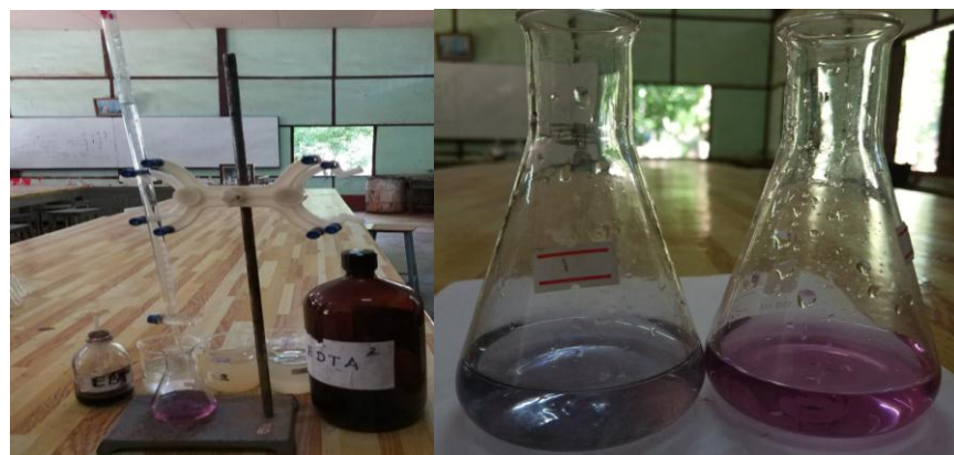
Figure 14 Determination of hardness of water samples by EDTA titration method (Before treatment)
