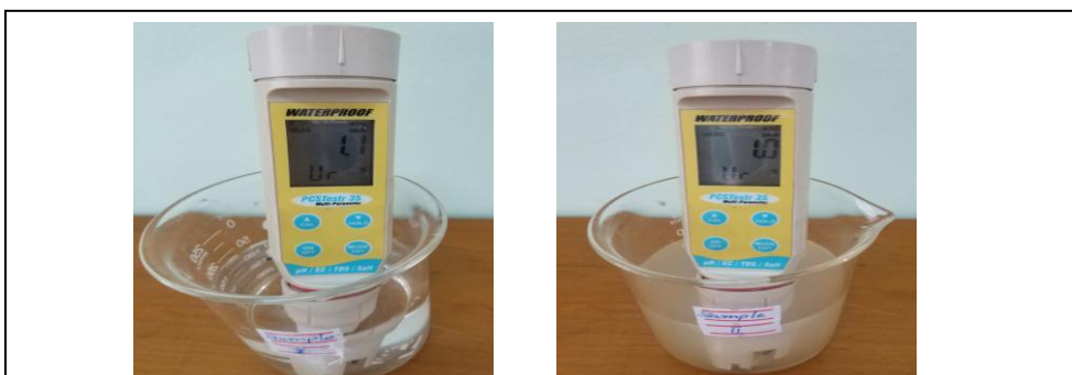
Figure 12 Total dissolved solids measurement of water samples by TDS meter (Before treatment)
