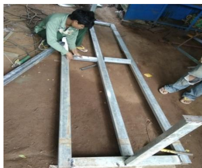
Fig.3.1.1 (b) Welding the parabolic skeleton of trough and base structure
