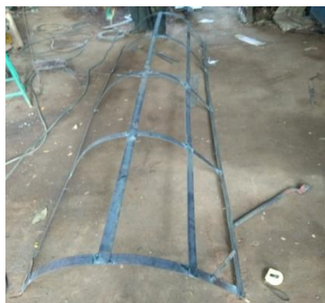
Fig.3.1.1 (b) Welding the parabolic skeleton of trough and base structure
