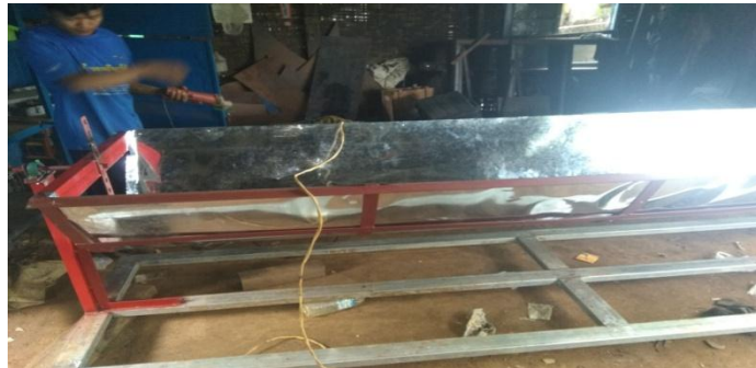
Fig.3.1.2 Arrangement of zinc sheet on the skeleton of collector
