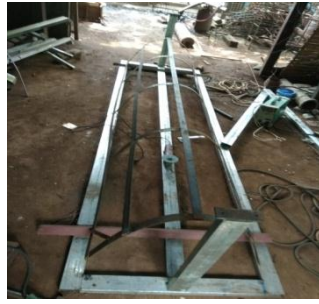
Fig.3.1.1 (c) Installation of skeleton of trough on base structure
