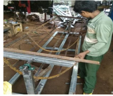
Fig.3.1.1 (c) Installation of skeleton of trough on base structure
