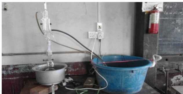
Figure 2- Extraction of fat from wheat powder by soxhlet apparatus
